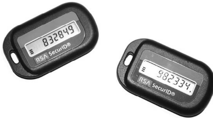
Figure 6.4: Physical tokens used for two-factor authentication.
