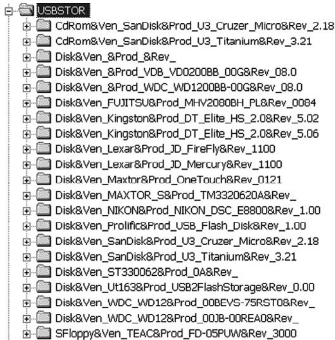
Figure 1.1: Identifying connected USB devices in the USBStor Registry key.
